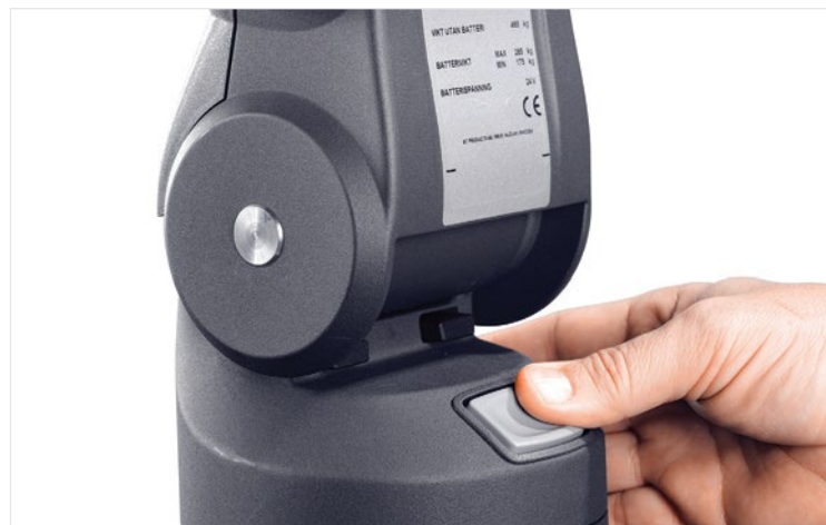
One-touch action to fold away the sideguards
